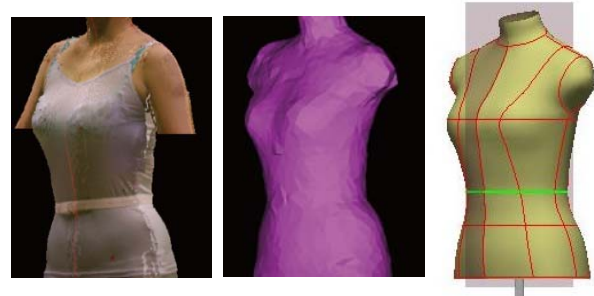
Fig. 2. The procedure of getting a subject's three-dimensional measured data as the digital virtual dress dummy of "lookStailor X".
