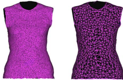
Fig. 1. The polygon data of a subject after cutting off the unnecessary area for analysis (left) and Homologous model of the same subject (right).
