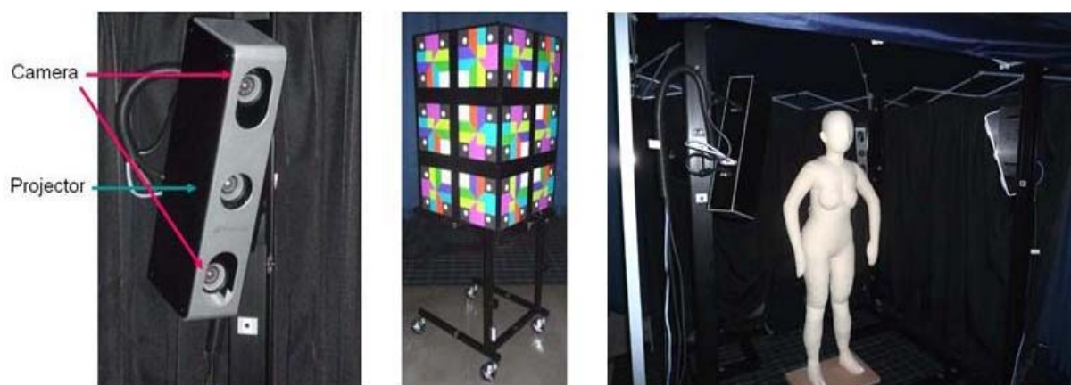
Fig. 1. Human Body Measurement System: Photographing Unit (Left), Calibration Box (Middle) and Whole System (Right)
