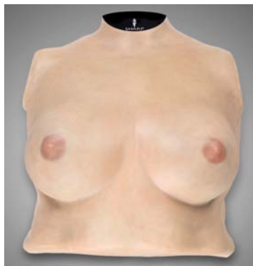
Fig. 6. Completed prototype manikin made from silicone skin, soft adipose tissue, rigid rib cage, nodular lumps and tumors.
