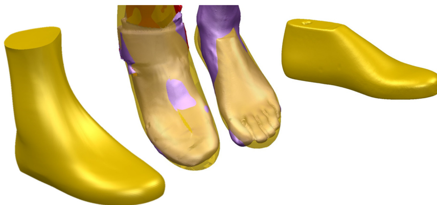
Fig. 10. From left to right: designed individual last, foot with orthosis and individual last, foot without orthosis with base last, and base last.
