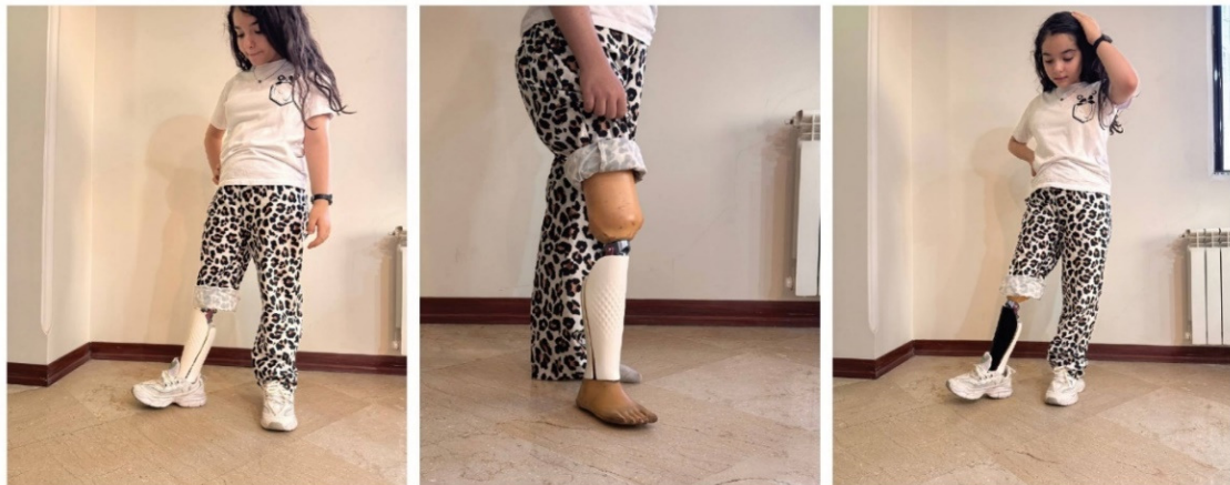
Fig. 13. Testing of 3D-printed prototypes and checking the dimensions and fitting of the cover with the prosthesis.
