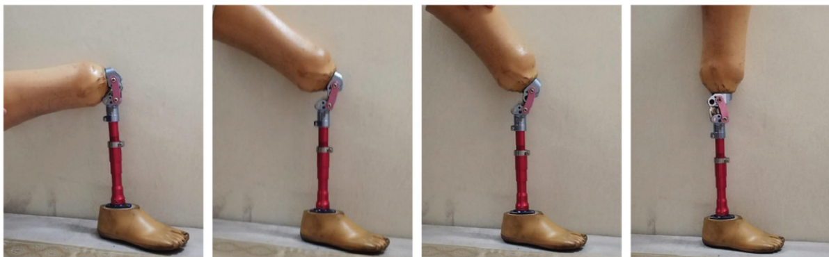
Fig. 4. Examination of different prosthesis angles to identify movement limitations.
