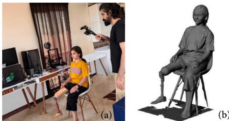
Fig. 2. (a) Process of 3D scanning, involving acquisition of geometric dimensions and point cloud; (b) Final model obtained from the scan and its meshing.
