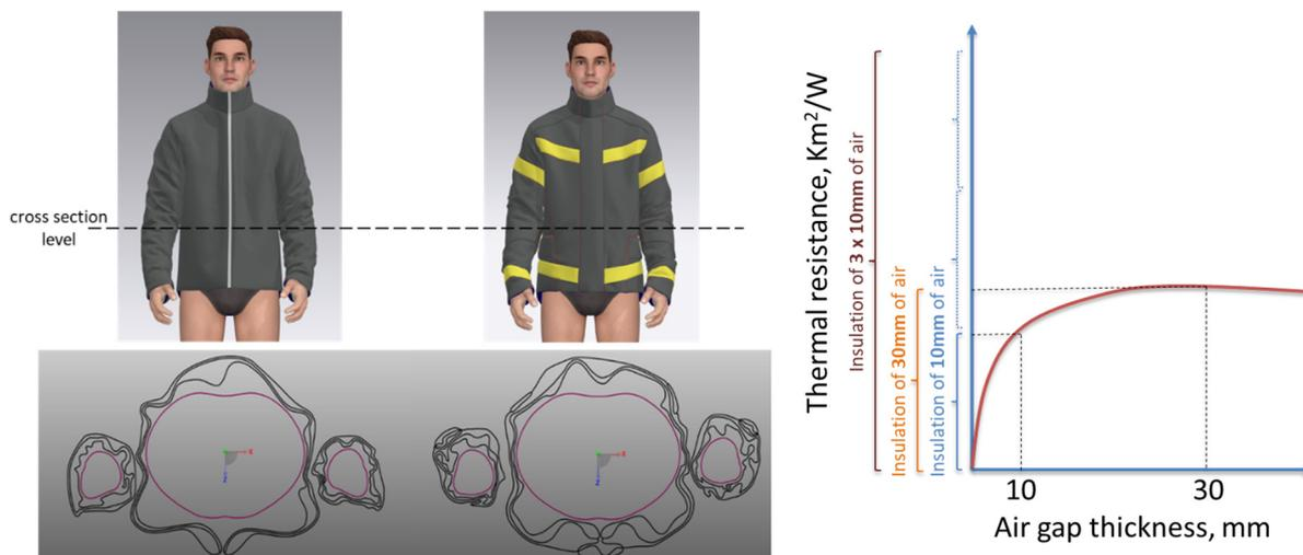
Figure 1. Visualisations and cross-sections of plain jacket and jacket with all construction details consisting of 3-layer fabric assembly (left), and principle of propagation of thermal insulation across enclosed air layers in clothing (right).
