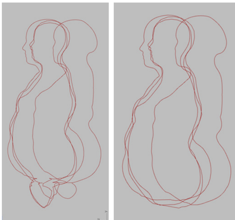
Figure 3: When thighs are touching during a scan, the result can be an incorrect projection of crotch point. Shown on left are uncorrected and overlaid outputs of the four mobile scans for one individual, participant 1002. The “bridging” of thigh data is evident. The right illustration shows corrected crotch points and crotch curves.
