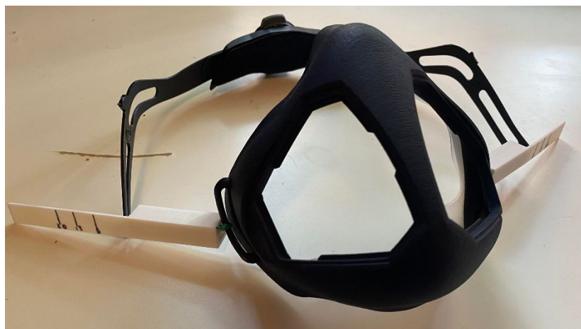
Fig. 4. Instrumented mask (without filter cartridges) for measuring tightening force. The bicycle helmet tightening device makes it easier to manage the tightening of the mask. When the mask is tightened, the springs on the sides (in the white rulers) will stretch and knowing the characteristics and the elongation, the return force of the spring can be deduced (which is equal to the tightening force).
