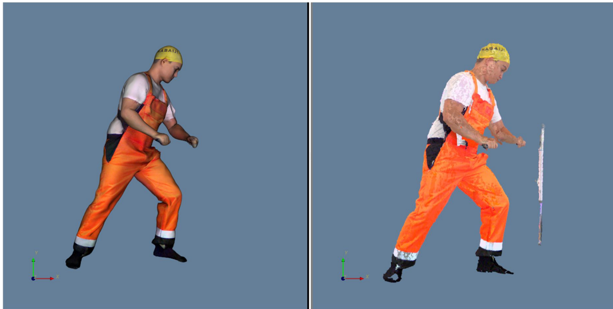
Fig. 5. Maritime worker recorded using a container lashing tool coated in shiny black, Dupli-color, 693854. Left shows a watertight and accurate homologous model of the human body. Right shows the raw data from one frame of the capture.
