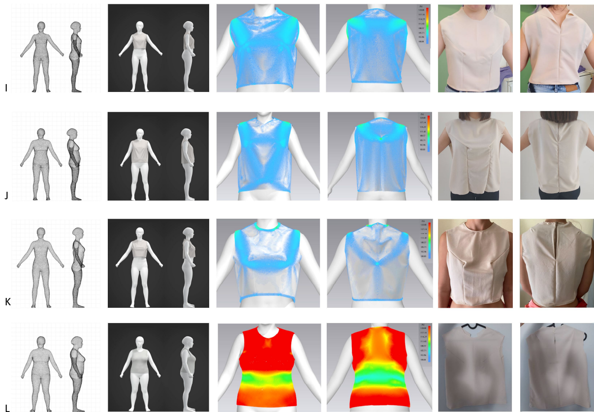
Fig. 5 2D body mesh (front-side), extracted obj in CLO, strain map on bodice, physical dressed bodice. (From left to right)
