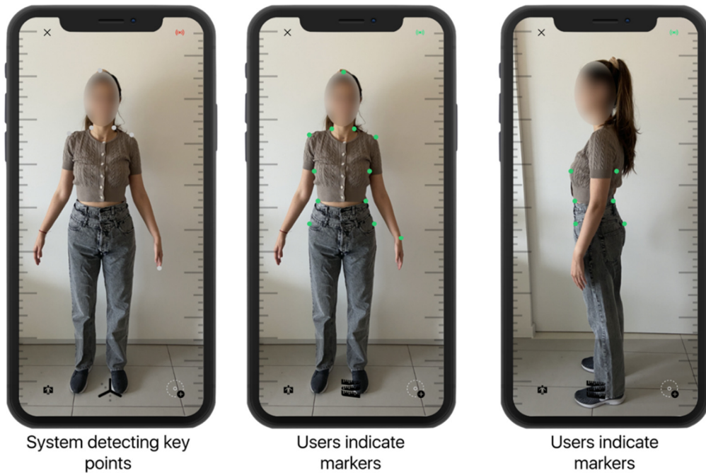
Figure 4: Indicating markers (semi-auto): Our advanced computer vision algorithms detect the dressed human body on 2D photos taken with any smartphone on any background and based on the detected body will indicate semi-auto markers. Users are also able to indicate their own markers.
