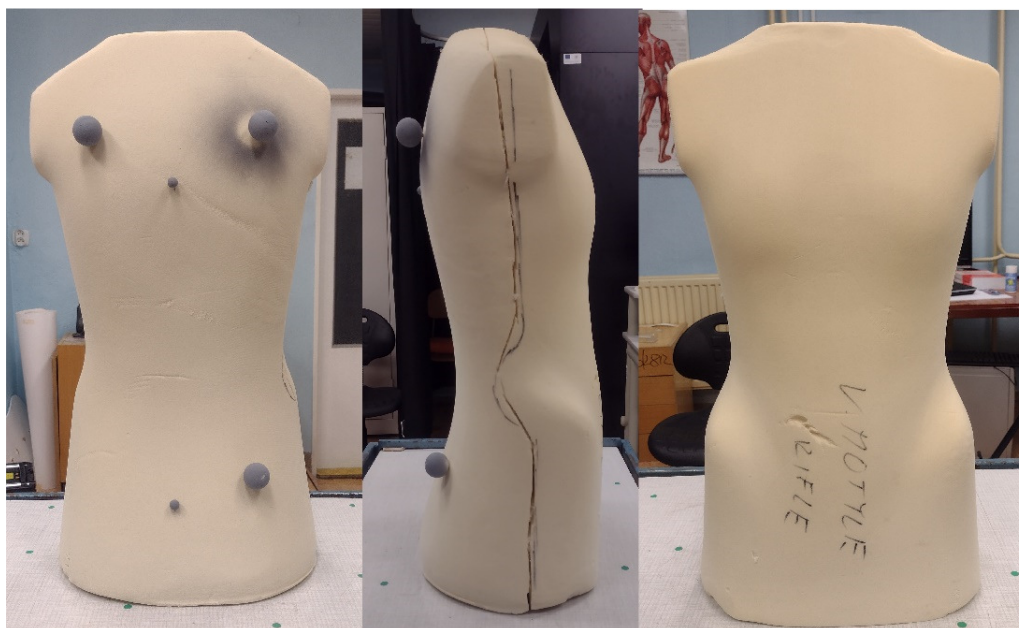
Fig. 1 A milled mold of the human torso with applied landmarks on the posterior side of the model
