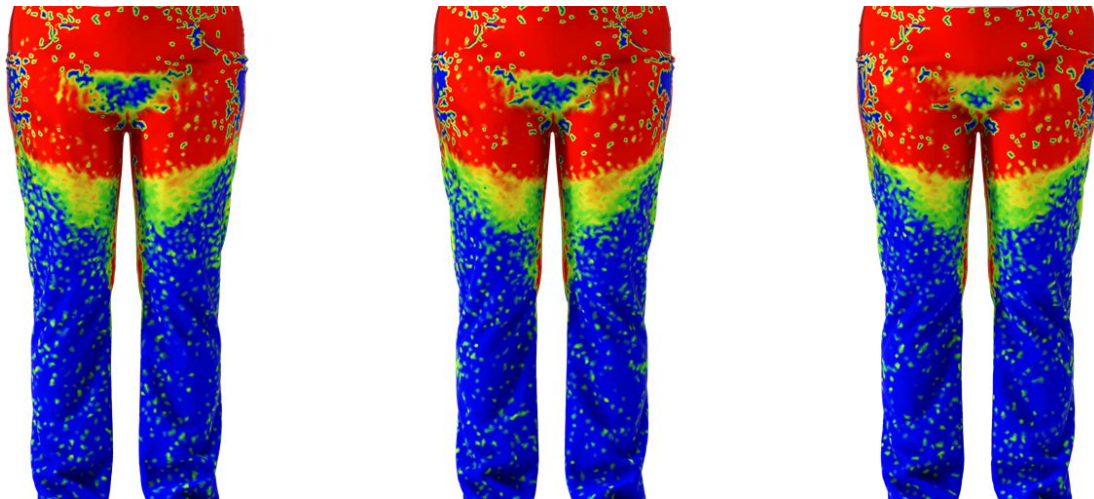
Fig. 8. Display of the tension map calculated in Vidya (f.l.t.r. LOD0, LOD1.3, LOD2.2)
