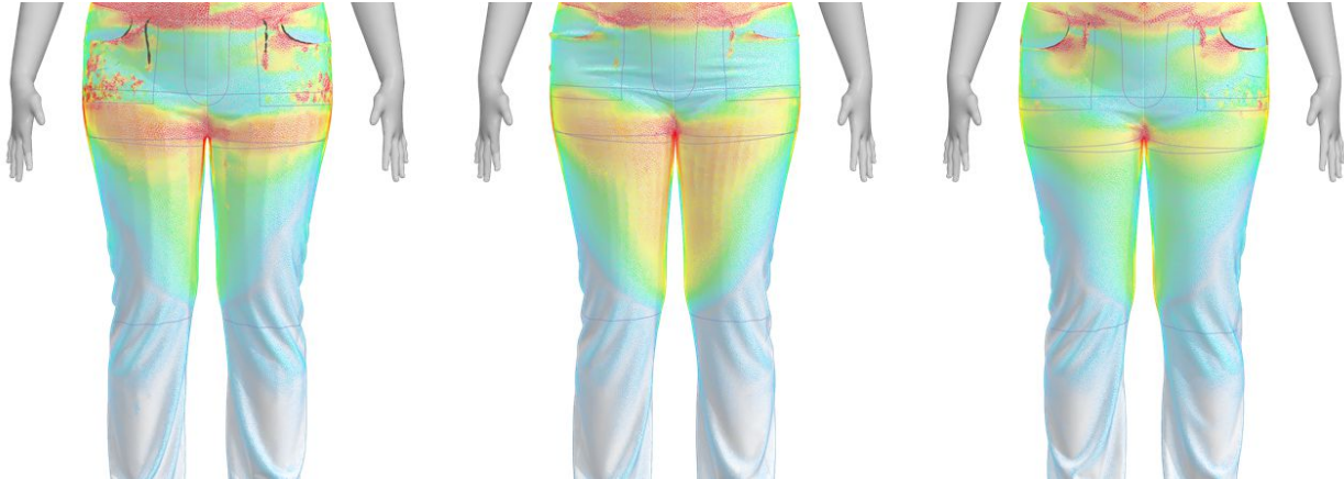
Fig. 6. Display of the tension map calculated in Clo3D (f.l.t.r. LOD0, LOD1.3, LOD2.2)
