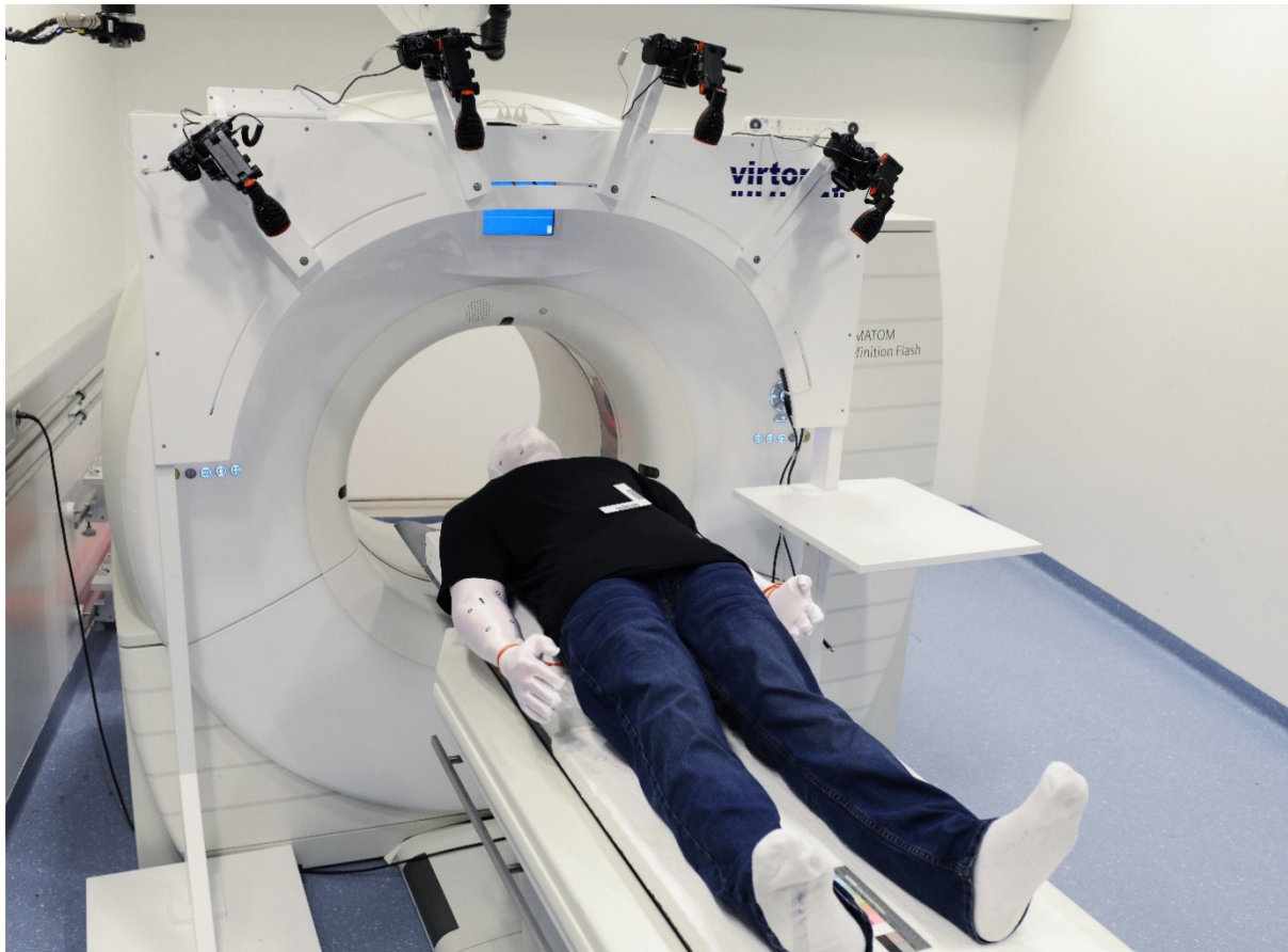
Fig. 1. Multispectral photogrammetry setup equipped with four modified DSLR cameras, NIR light sources, IR longpass filters and remote shutter controls. The setup is placed in front of a CT gantry and aligned centrally above a dressed mannequin.
