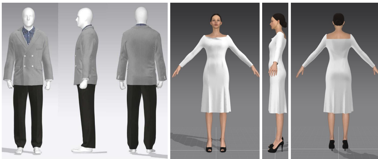
Fig. 4. An automatically generated standard set of garments for a statistical avatar and a Made to Measure set of garments for a customer-specific avatar. (ELSE-Corp, Savitude)
