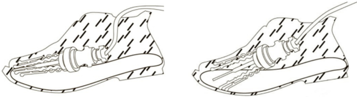
Fig. 3. Scanning process of the inner surface of the footwear with probes in the retracted and opened position
