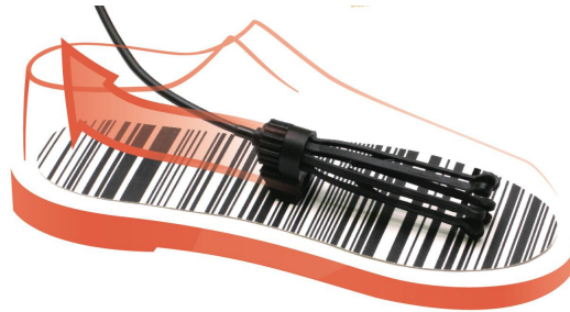
Fig. 1. Scanning process of the inner surface of footwear performed with the FITT™ Scope
