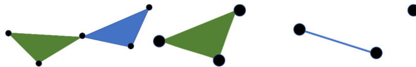
Fig. 7. Geometry with missing connectivity – not enough connected surfaces, single face or single edges and points
