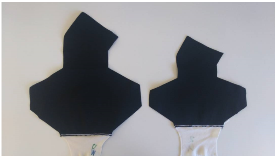
Fig. 10: Test swatches to determine stitch parameters. Swatches based on the same geometry, knit with the same arbitrary stitch parameters, but with different stitch constructions, differ significantly.
