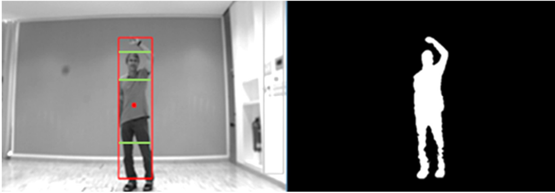
Fig. 2. Acting person with detected body areas (left) and extracted blobs (white region - right)
