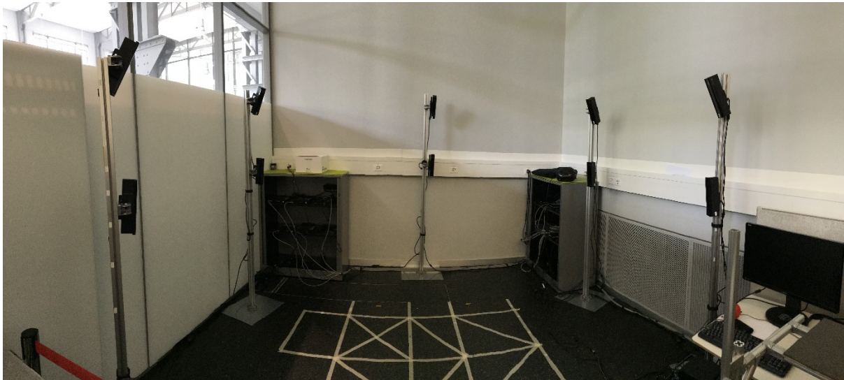
Fig. 5. Configuration of the 10 Kinect v2 in the room (facing inward configuration)
