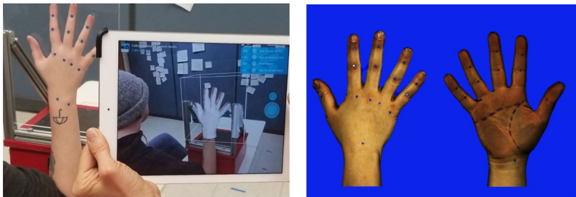
Fig. 2. 3D hand scanning process with Occipital Structure sensor
