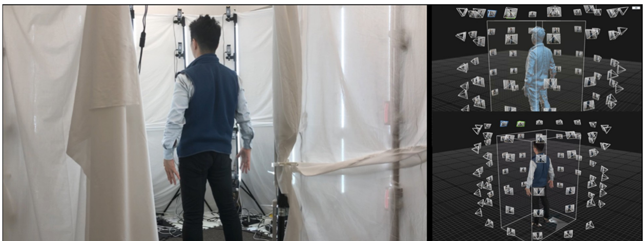
Fig. 1. A human subject surrounded by 88 units of Raspberry Pi Zero W + Camera Module and processed in photogrammetry software, RealityCapture [3]. The number of camera units vary from 80 to 112.
