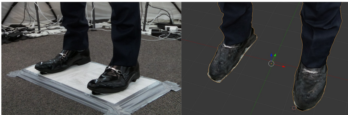
Fig. 14. The surface mesh of the black shiny shoes isn't reconstructed properly
