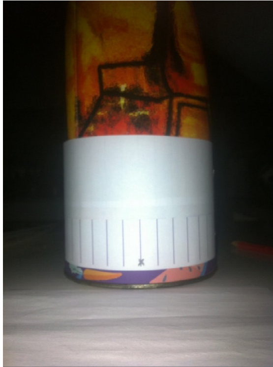
Fig. 4. Flash photograph image of paper covered cylinder, after reduction to 108 columns x 144 rows. The cylinder is marked with lines at 10 mm spacing.
