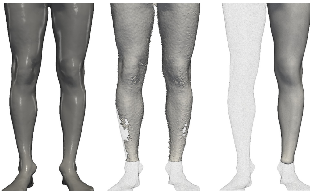
Figure 3. A baseline scan (left), one raw scan generated from the baseline scan (middle) and its reconstruction using Shapeshift 3D Repair™(right).
