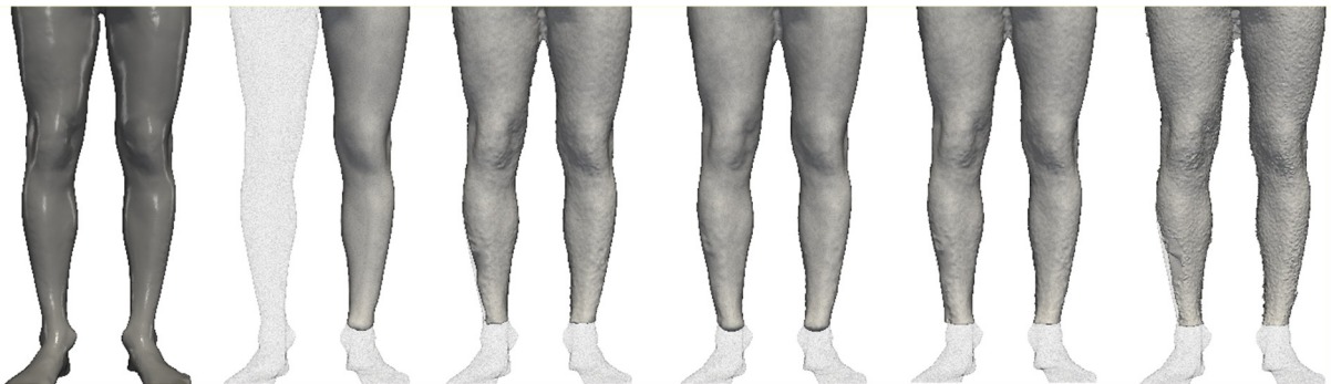
Figure 5. Baseline scan of the left leg (left) and the related reconstruction from ShapeShift 3D Repair™, Dirichlet-Poisson, Free-Poisson, Neumann-Poisson and Power Crust methods in order, from left to right.
