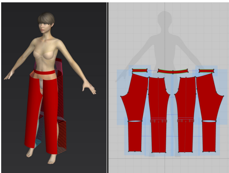
Fig. 2. Assembly process of the prototype with virtual sewing.
