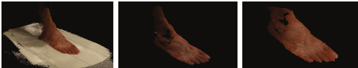
Fig. 2. (a) Point cloud acquired by smartphone depth camera; (b) after removing plane; (c) after filtering and extracting foot shape
