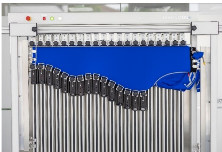
Fig. 2. HOSY test of pressure gradient of functional t-shirt
