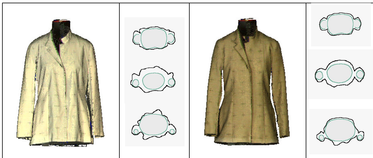
Fig. 1. Scans of test garments in German size 38 (bust girth 88cm) with differing widths, cross sections at bust girth, waist girth and hip girth (top down) to investigate distances and contact areas
