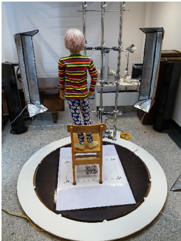
Fig. 5. 3D rotary scanning system
