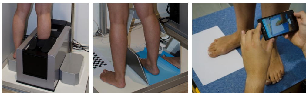
Fig. 8. Digital acquisition of 3D feet, from left to right: Infoot, DomeScan, Avatar3D app.
