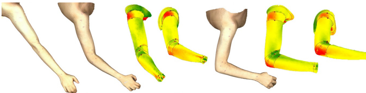
Fig. 10. Application of the same algorithm for the analysis of the upper limbs. Red and green areas indicate the parts of stretching and compression of the skin during the bending of the arm.
