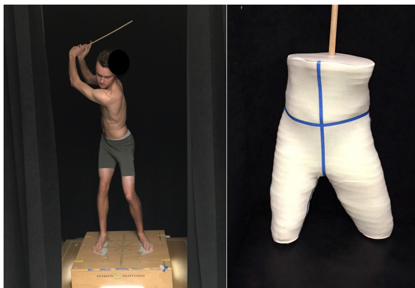
Fig. 3. Half scale form developed from the scan in the golf swing pose
