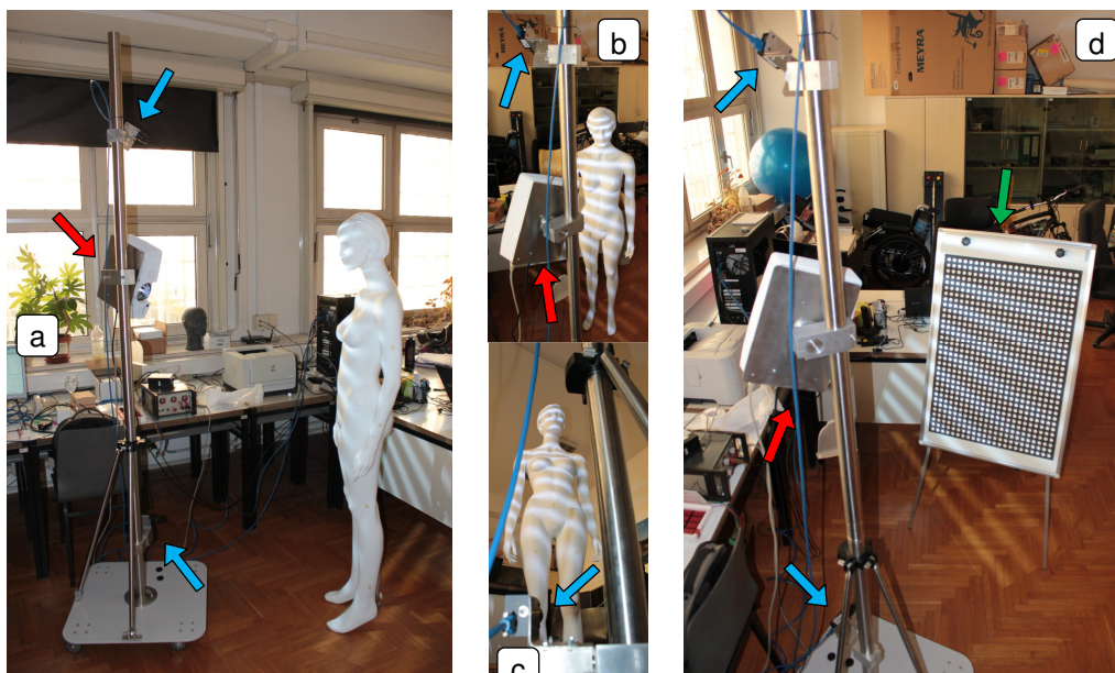
Figure 3. Prototype of a low-cost 3D human body scanner: (a) side view; (b) top camera; (c) bottom camera; (d) back view showing a calibration board. Arrow indicators: cameras are blue, projector is red, and calibration board is green.
