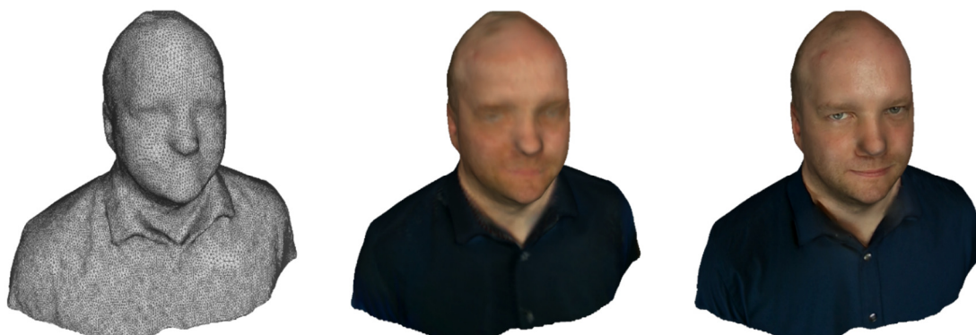
Figure 1 Comparison of vertex coloring and texture mapping. Left: Wireframe of model consisting of 70k vertices. Middle: Vertex colored version using 70k vertices. Right: Texture mapped version using 10k vertices.
