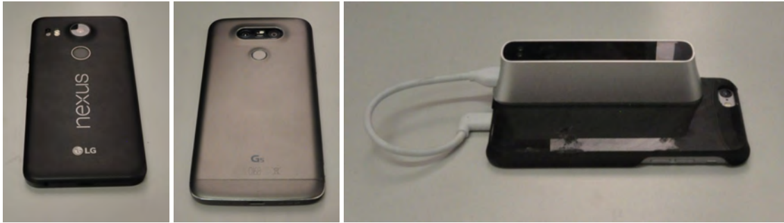
Figure 2: Hardware used to capture the data. Left most the monocular camera, a Nexus 5X phone. Center, the LG G5 phone with a stereo camera setup. Right most, the iPhone 6 with the additional Structure IO sensor.
