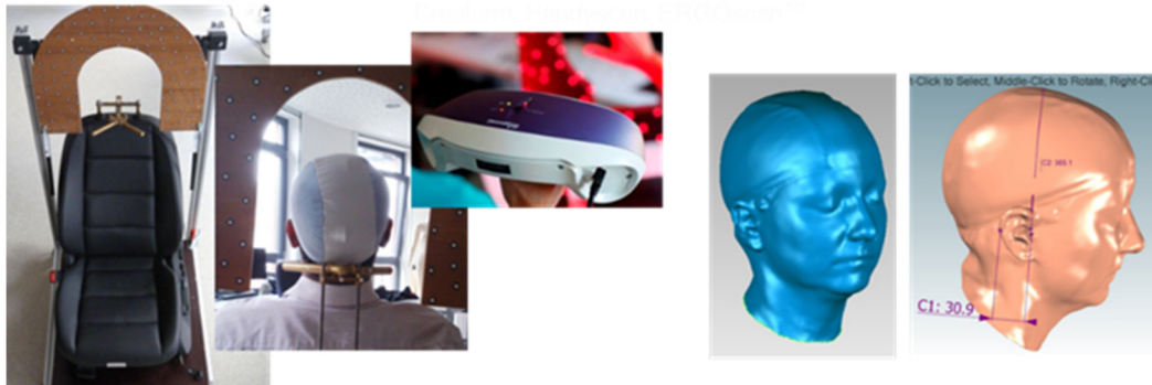
Fig. 3. 3D head scanning process with Creaform Ergo Handyscan
