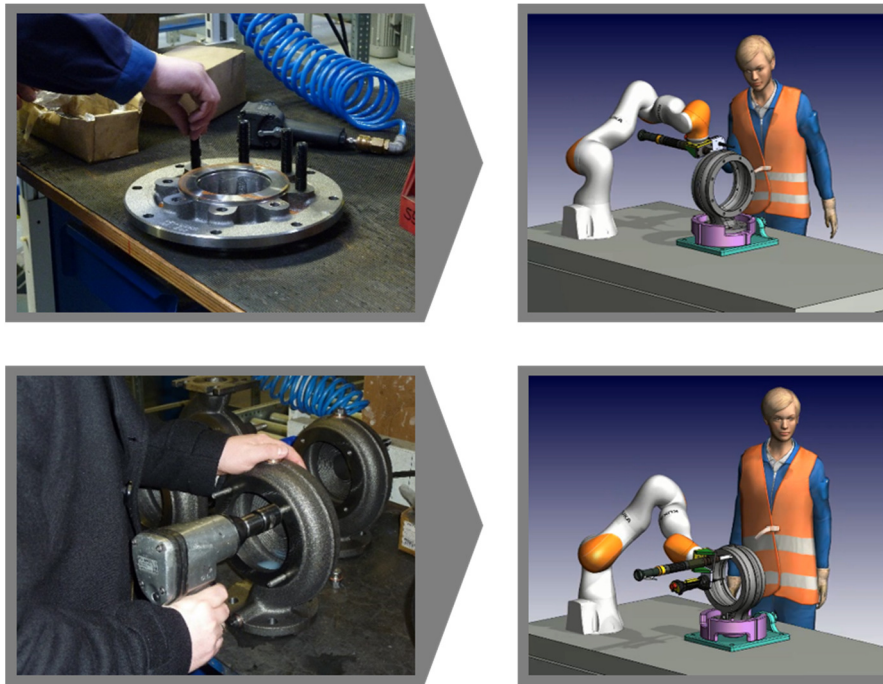
Fig. 1. Assembly of Stud Screws (left: current process, right: plant assisting process)
