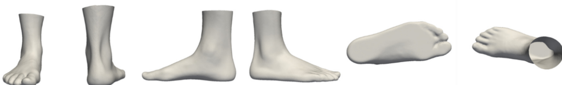
Fig. 7. A normalized 3D flat foot model (mean foot length 264.7 mm) obtained using similarity alignment
