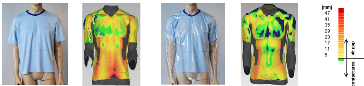
Figure 1. Photographs and corresponding post-processed exemplary 3D scans indicating the contact area and the air gap thickness of the loose-fitting inner layer alone and in combination with the outer layer jacket.
