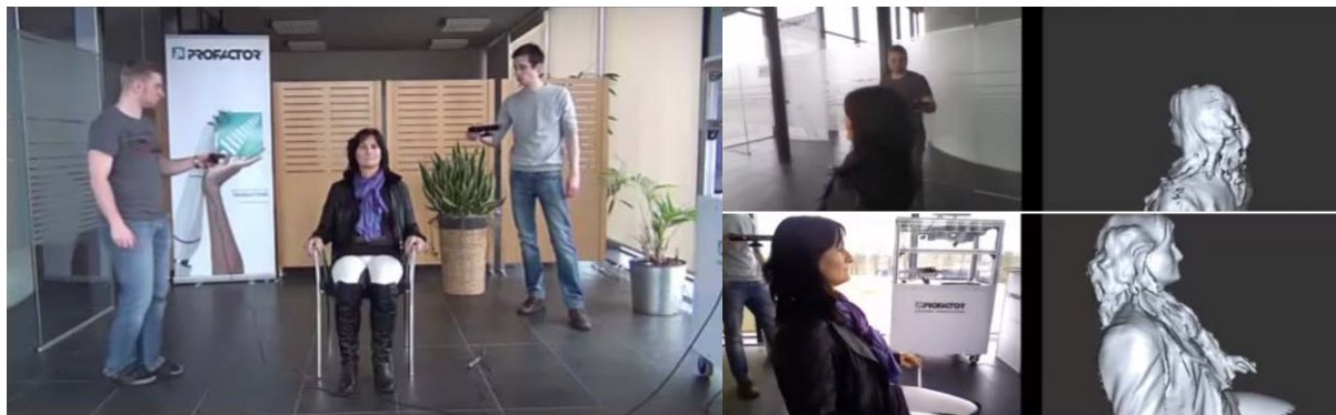
Figure 2 Multi-sensor cooperative reconstruction. Left: Image of setup. Top-right: first sensor. Bottom-right: second sensor.
