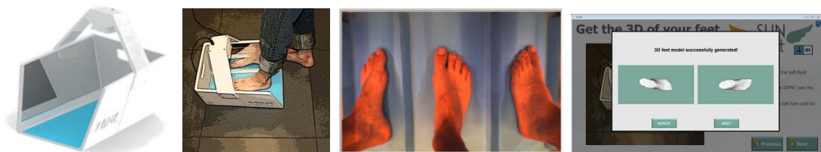
Fig. 6. Booth setting, one-shot scanning process, single image and resulting feet
