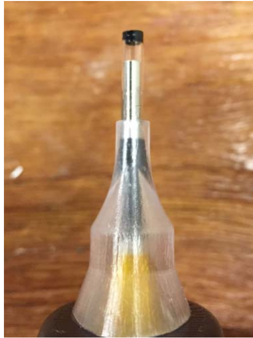
Figure 2. Distal end of the eFit scanner shows the cylindrical light guide, the distal end of the center camera optics, and the sectioned cylindrical dichroic cone
