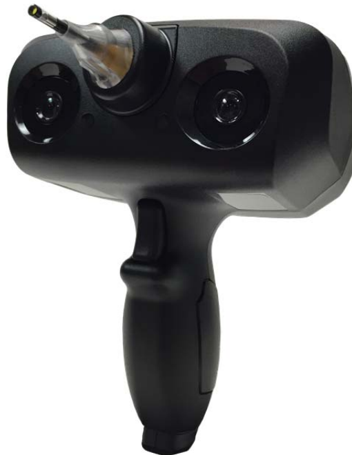
Figure 1. The eFit 3D ear scanner includes a radial 3D scanner for the ear canal and under cuts in the pinna, a line scanner for the flat regions of the pinna, two tracking cameras, a video otoscope, and an integrated LCD.
