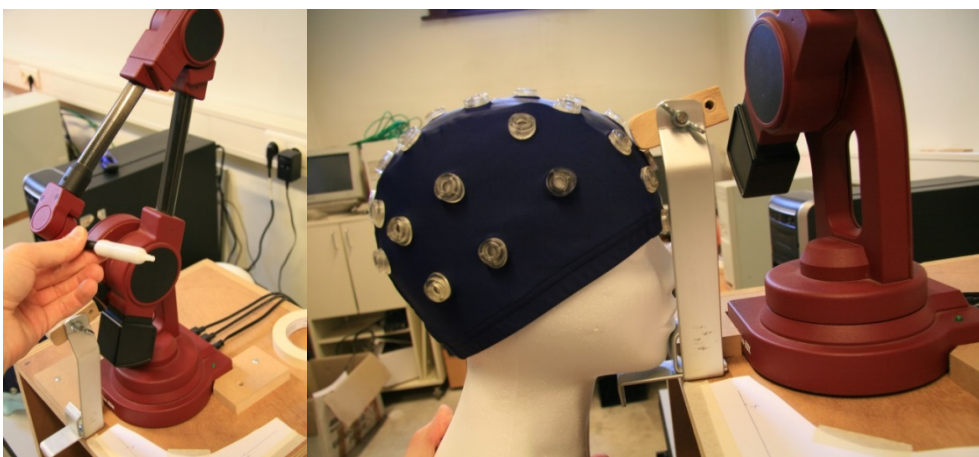
Fig 4: Measuring setup with the digitizer, the head fixture and cap on a (smaller than regular) foam head model.
