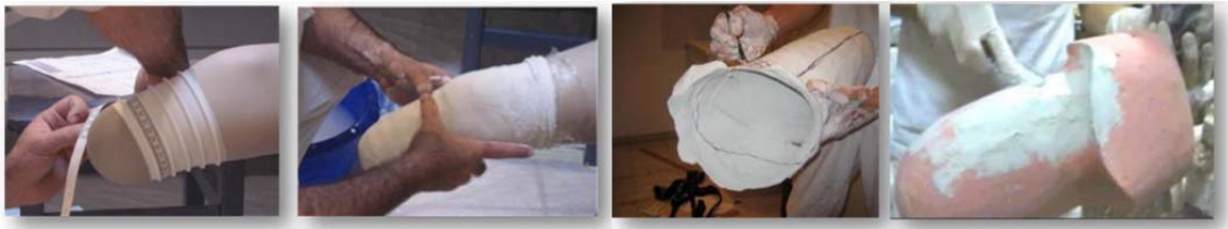
Figure 1 - Traditional socket development process
