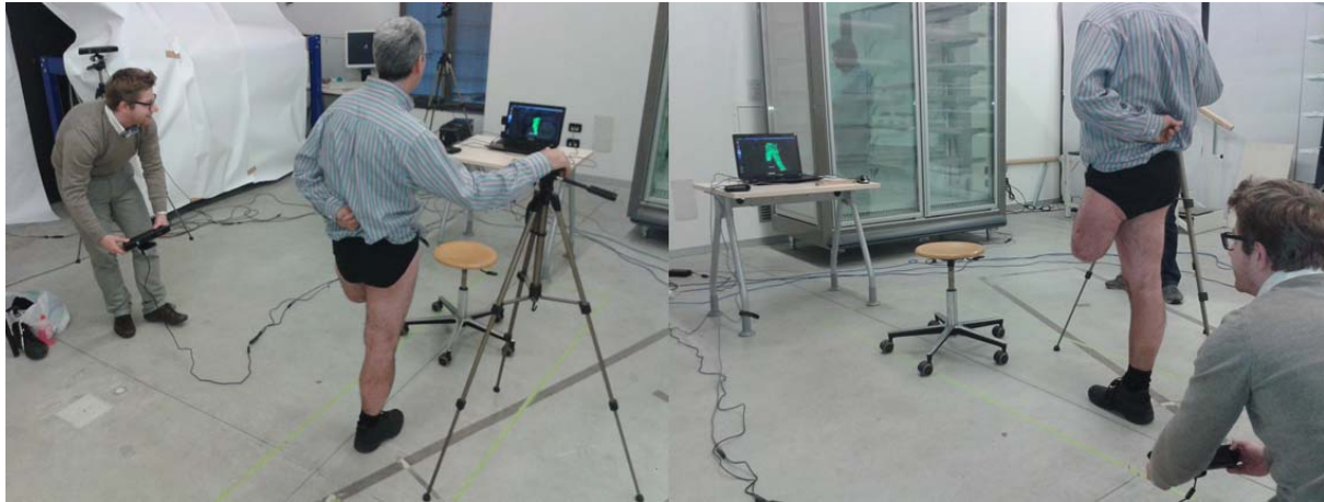
Figure 6 - 3D scanning procedure of a lower limb patient with MS Kinect v1
