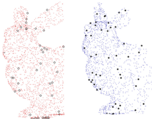
Fig. 4. Corresponding points from curvedness algorithm by [9]; although views have significant overlap, wrong points are selected as correspondences.
