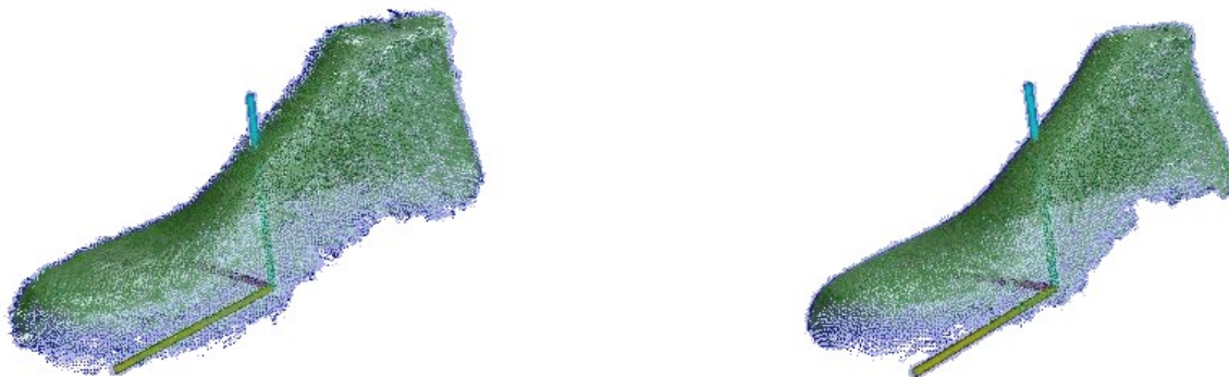
Figure 5: Left: raw point cloud with floor removed and (right) cleaned point cloud
