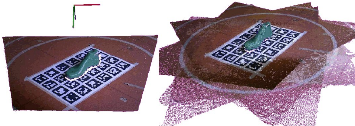
Figure 5: Left: Single view captured with the grabber (point cloud+texture) and (right) single point cloud obtained from multiple view registration (8 in this case)
