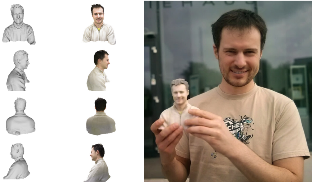
Fig. 4 Left, 3D bust model. Right, printed 3D bust.
