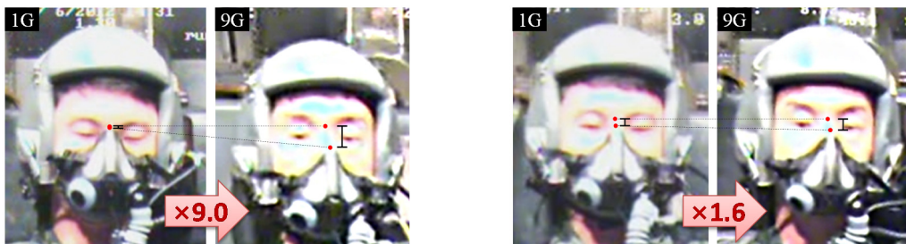
(a) Existing oxygen mask (b) Revised oxygen mask Fig. 14. Video analysis results (illustrated)
