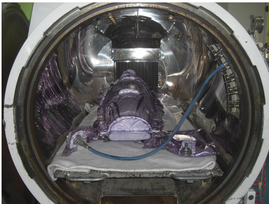
Fig. 8. Autoclave for the carbon fiber polymerization process.
