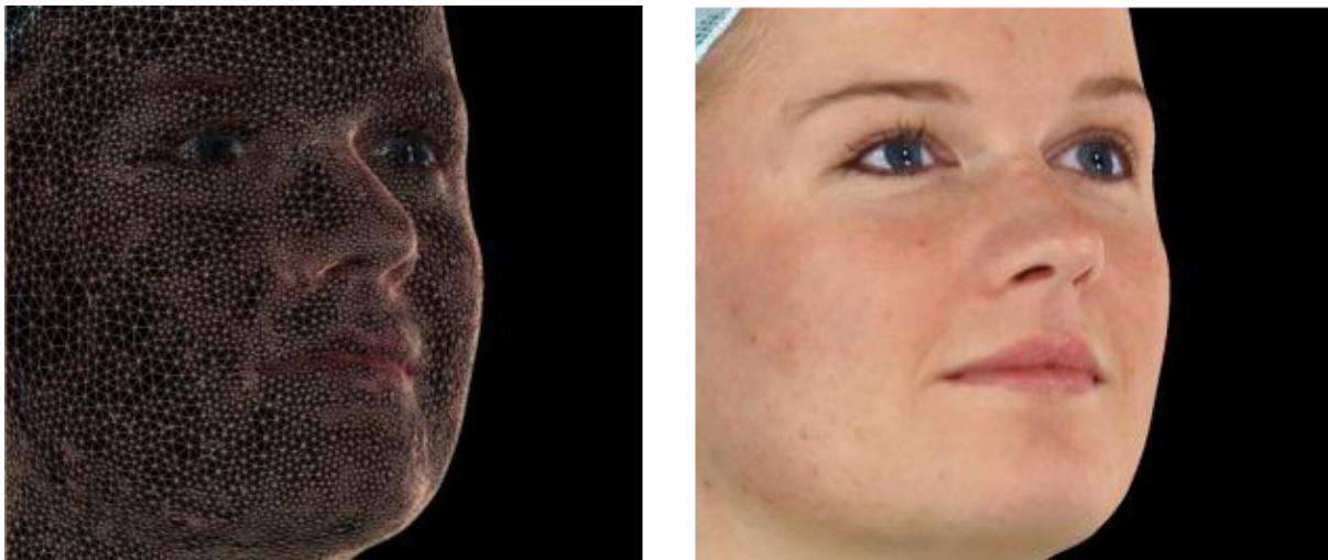
Fig. 9. Final mesh with curvature dependent density (left) and with texture (right).
