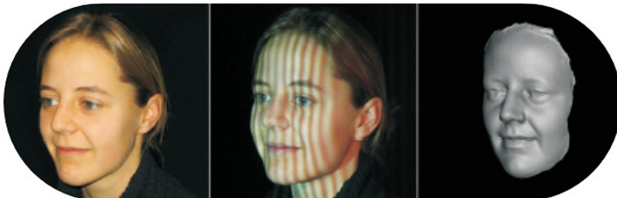
Fig. 4. Acquisition of a single 3d view.
