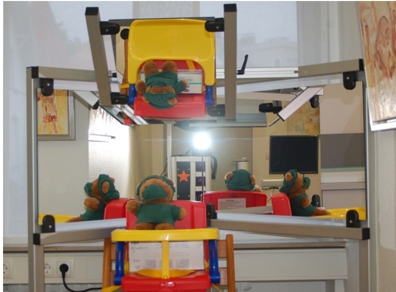
Fig. 15. Four-mirror setup to get 5 views with one shot.
