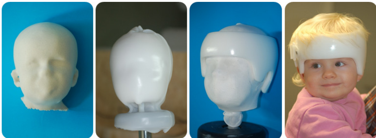
Fig. 16. Manufacturing the helmet by rapid prototyping.
