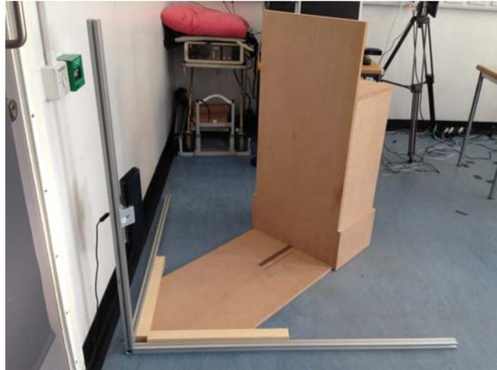
*Fig. 3. Kinect calibration rig.*
